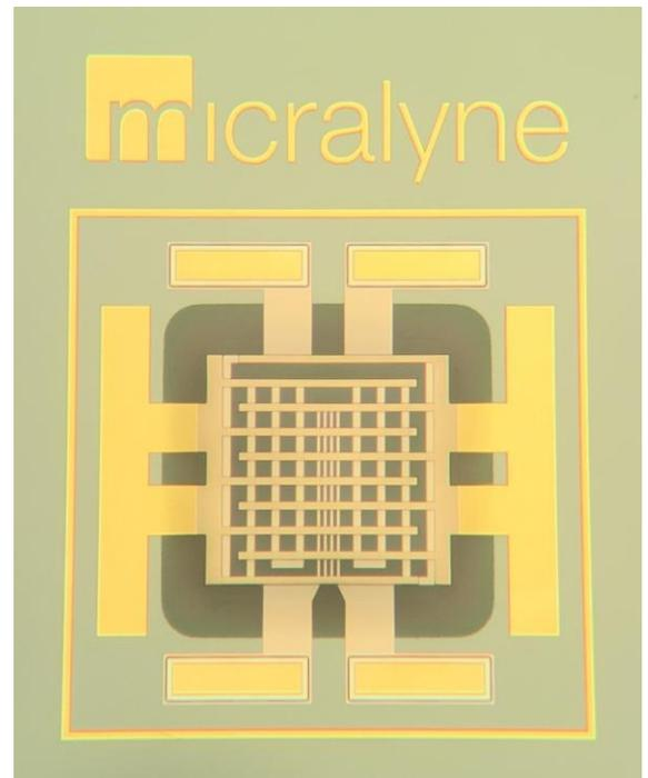
**Figure 1: Metal Oxide Gas Sensor with integrated micro hotplate, 1.6mmX1.6mm die size**
